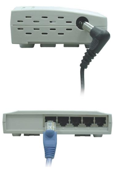
Power is supplied through an external DC power adapter. Check the technical specification section for information about the DC power input voltage. Since the switch does not include a power switch, plugging its power adapter into a power outlet will immediately power it on.
